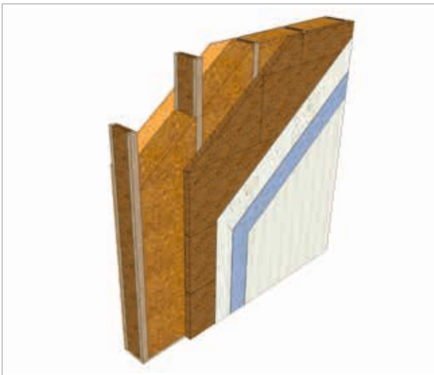
Timber frame with no external board material
